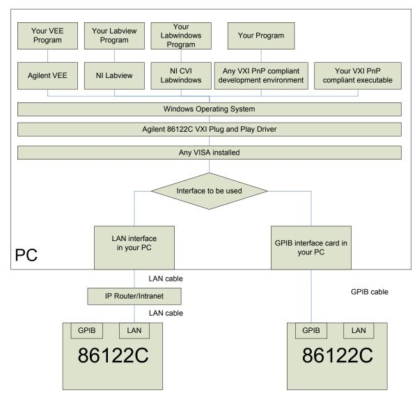
Controlling the 86122C using the 8612x VXI Plug and Play driver
