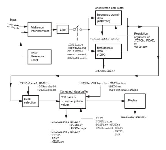
After collecting the uncorrected data, the Agilent 86122C searches the data for the first 1000 peak responses.
